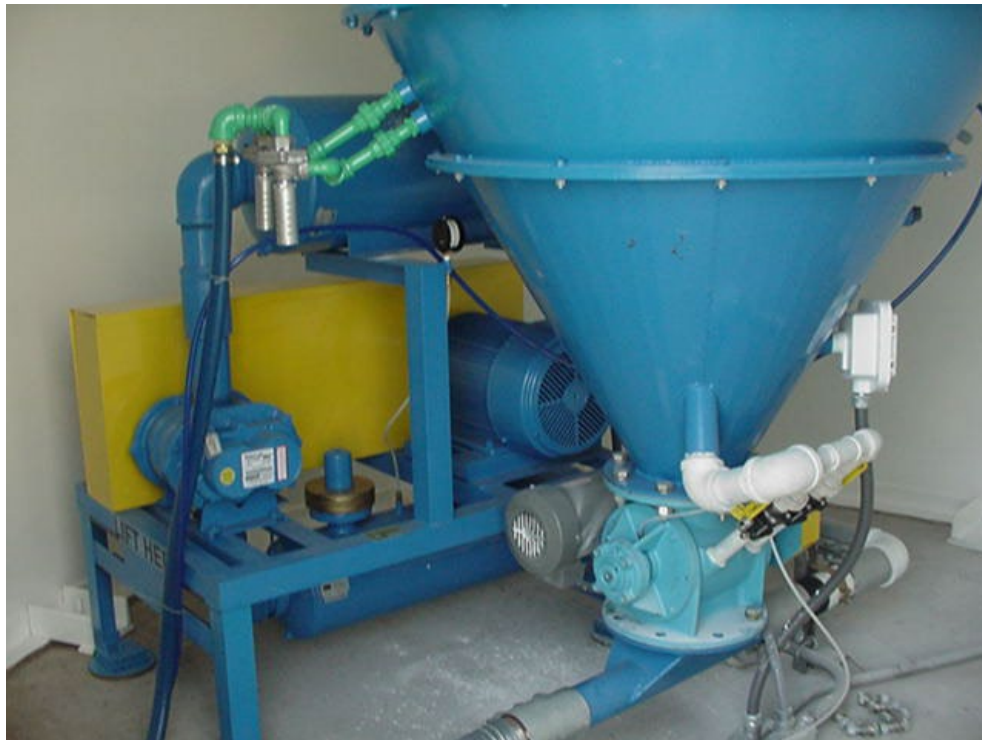
Cone Valve Discharger No flex sleeve, totally sealed
