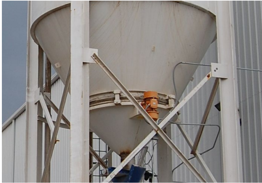
Standard Bin Activator with Flex Sleeve
